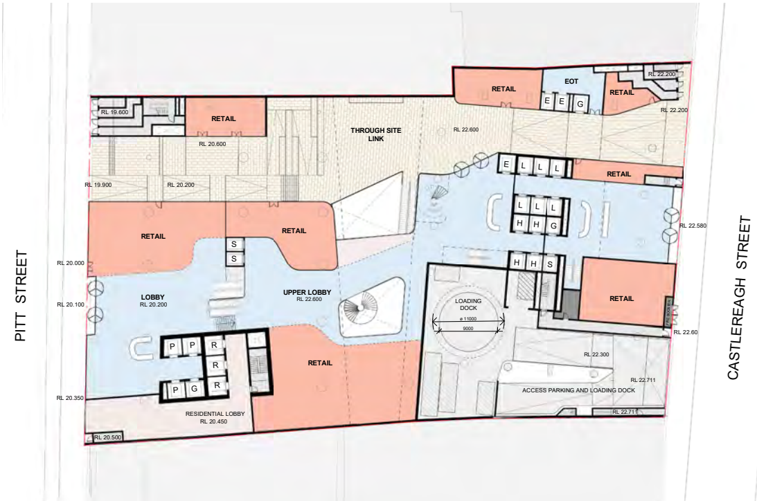
Ground - MRV and SRV Loading Dock
